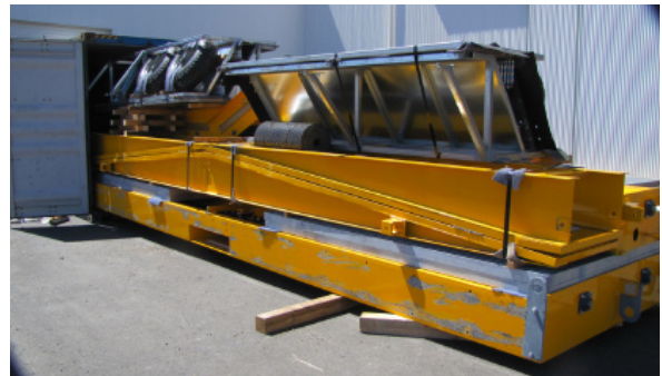
Caption: One of the purpose-built Famson Drive Over Hoppers is dismantled and packed for shipment to South Africa.
